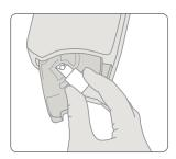
Place microcuvette into analyzer.
